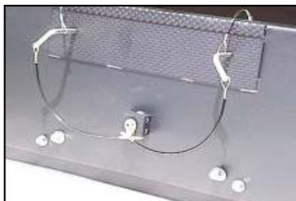
The *Motor Positioning Pins* are secured to the **Cap** and assist in the rapid lock-in of the Johnson **Enforcer** 55HP motor to the transom, through the use of matched pre-drilled alignment holes.
