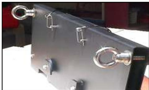
The **Cap** is fitted with two large, easy to use, utility *Eyebolts*. They are particularly handy for use as tie down points, towing bridal hook up or as aft lifting points for the craft.
